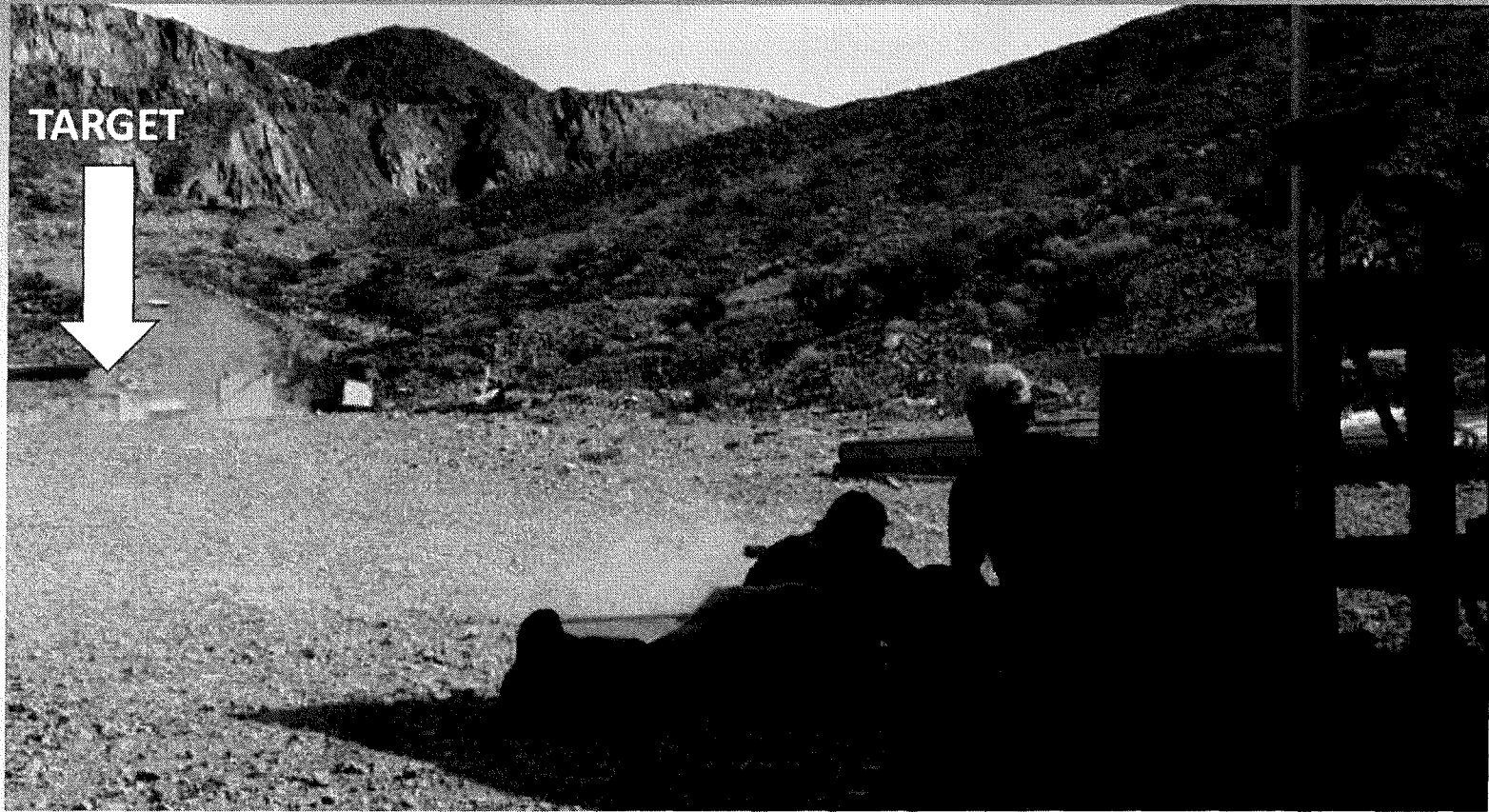
US Ranger shooter fires .50 caliber BMG ammo at safe door filled with BallistiCrete. Distance to target, 50 yards.
